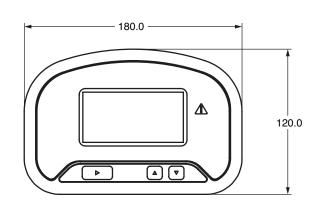
Recommended panel cutout: 92 (+0.8,-0) x 138 (+1.0,-0)mm Acceptable panel thickness (snap-fit fingers): 0.8 to 3.8mm Acceptable panel thickness (bracket): 5.0 to 8.9mm
